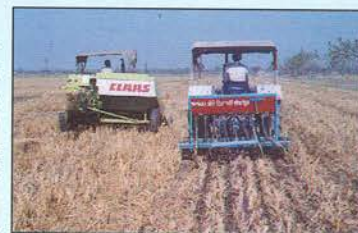
Pant Zero-Till Ferti-Seed Drill developed by Pantvarsity has become very popular in rice-wheat system of north India
