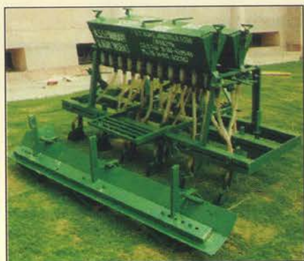
New zero-till cum bed planter with the shaper placed in front of it
